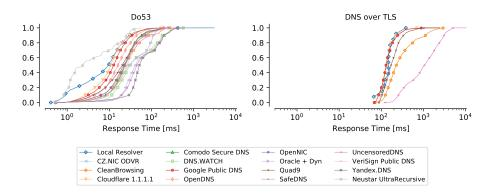
**Fig. 3.** CDF of resolver response time for successful Do53 (left) and DoT (right) requests (5<sup>th</sup> percentiles per probe). While most Do53 responses arrive within roughly 100 ms, the majority of DoT responses require more than 100 ms to return.
