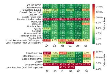
Fig. 1. Failure rates of resolvers by continent for Do53 (top) and DoT (bottom). Each cell represents the failure rate based on all failures relative to all queries for the specific resolver and continent. Most failure rates for Do53 are between 0.3–3%, whereas DoT failure rates are generally higher and more varying.
