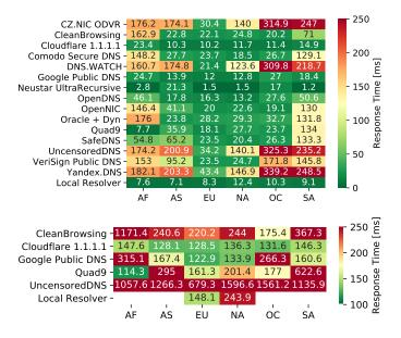
**Fig. 4.** Medians of the 5<sup>th</sup> percentile response times by continent and resolver for Do53 (top) and DoT (bottom). Do53 response times are mostly below 20–40 ms for most resolvers, whereas DoT response times are between roughly 120–180 ms instead.
