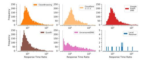
**Fig. 2.** Histograms of response time ratios (DoT to Do53) per probe for each resolver. The vertical dashed line represents the ratio of 4 RTTs for DoT (TCP handshake + TLS handshake + DNS lookup) to 1 RTT of Do53 (DNS lookup).
